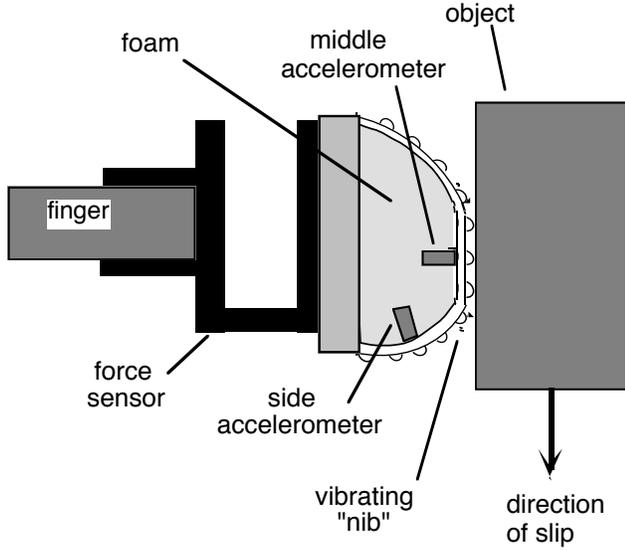
Figure 1. Cross-section of fingertip with dynamic tactile sensors on and off the contact area.
