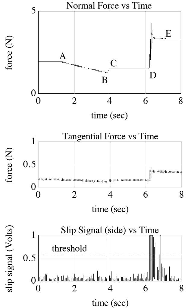
Figure 2. Plots of normal (grasp) and tangential (load) force for a fingertip holding an object, along with the signal from a side-mounted skin acceleration sensor during an incipient slip event and a disturbance in the load force.
