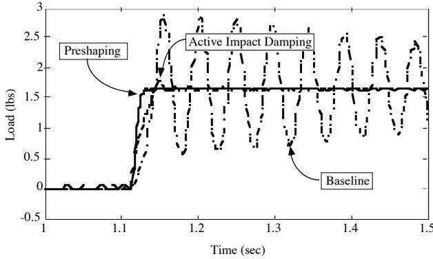
Figure 4. Force trajectory for fingertip contacting a hard surface: The effects of active impact damping [Khatib and Burdick 1986] and command input shaping [Hyde and Cutkosky 1993] are illustrated. Both methods greatly reduce the oscillations as compared to a simple baseline force control law, with the input shaping showing a slight advantage in rise time and overshoot.
