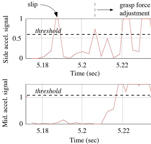
Figure 3. Comparisons of the signals from side and middle accelerometers (off and on the contact area, respectively) during an incipient slip and subsequent grasp force adjustment.
