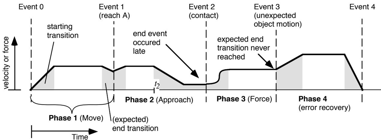
Figure 5. The Phase/Transition/Event sequence for part of a task is shown schematically above. Each phase begins and ends with an event such as fingers making contact or arriving at a specified location. In this example a fingertip approaches and touches an object, which slips unexpectedly.
