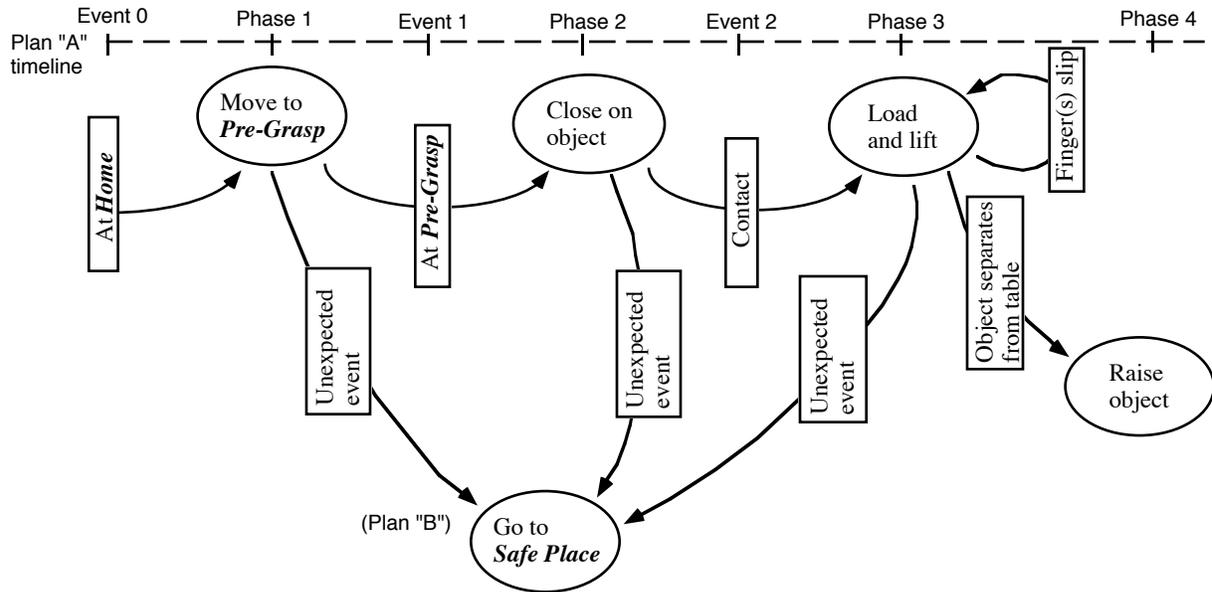
Figure 6. A fragment of a very simple plan for grasping an object. In the nominal plan, each phase (nodes in ovals) ends with an expected event (arcs with box labels). In this simple example, any event other than the expected (goal) event for each phase results in failure and retreat (Plan "B")
