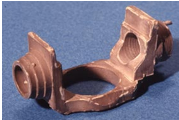
Figure 2-3: Sintered silicon nitride pitch shaft
