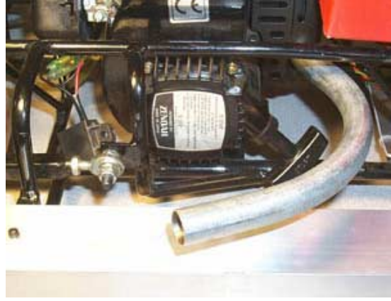
Custom-made exhaust pipe.
