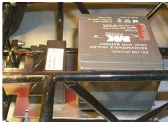
Yaw rate sensor and battery attached to aluminum plate.
