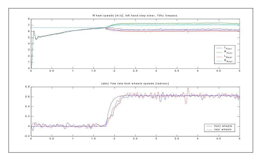
This figure represents a step steer of about 18 degrees in a Ford Winstar at just under 7 m/s on dry pavement. The solid lines are simulation results from the 4-wheel model and the dotted lines are low-pass filtered data from the ABS sensors.
