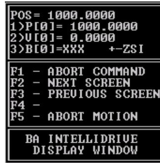
Figure 3-15. Teach Screen for Position “0” (Showing Current Position and Teach, POS, VEL, and I/O Pattern)
