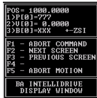
Figure 3-16. Teach Screen for Position “0” (Showing Current Position and Teach, POS, VEL, and I/O Pattern)
