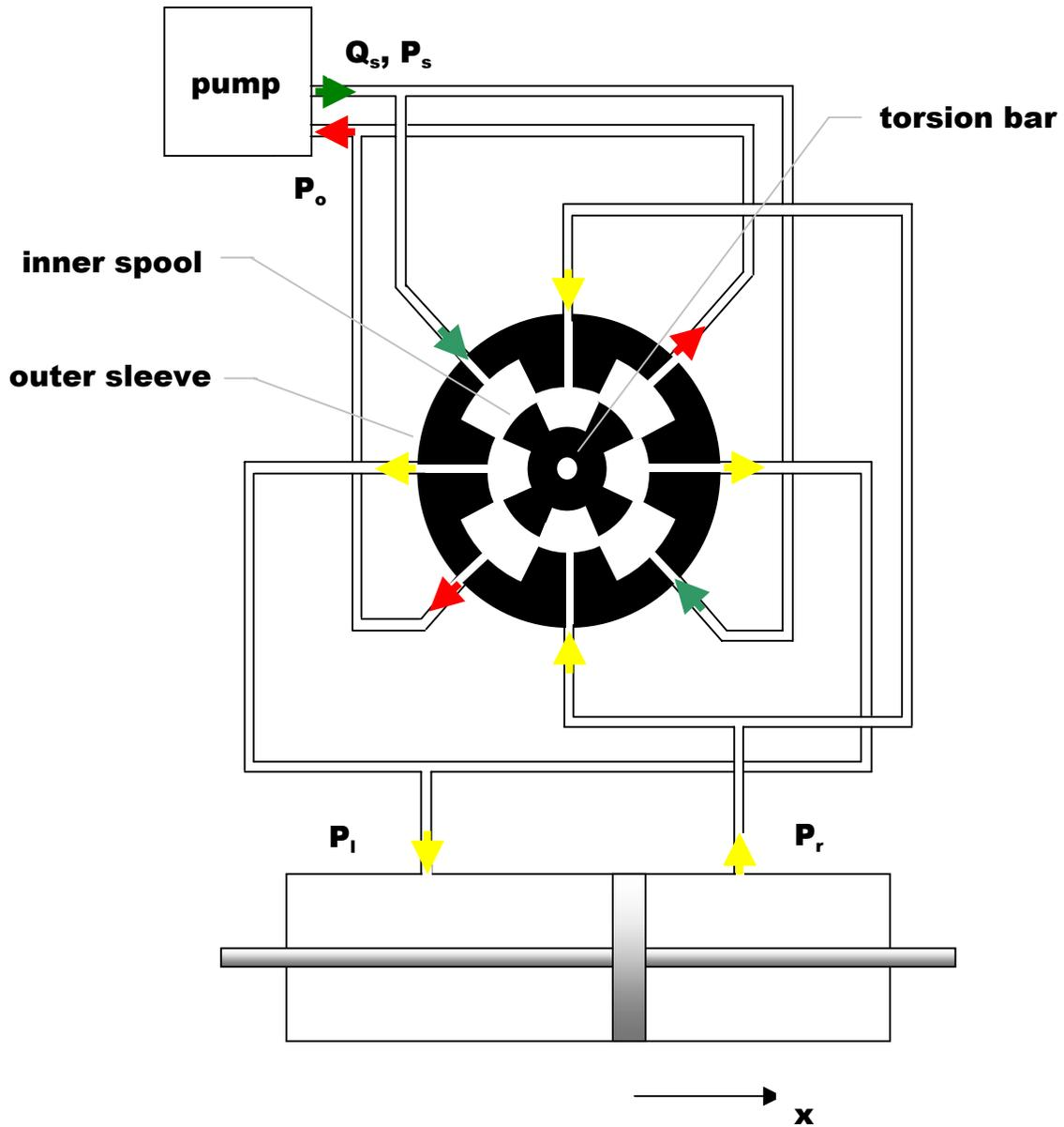
Figure 4: Hydraulic power assist schematic.
