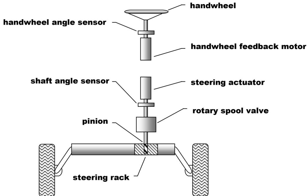
Figure 1: Steer-by-wire schematic.
