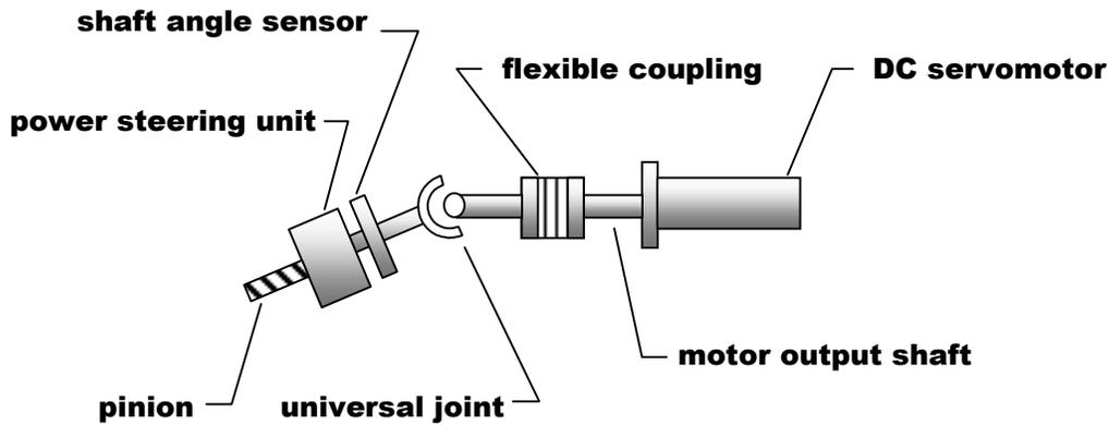
Figure 2: Steering actuation system side view.
