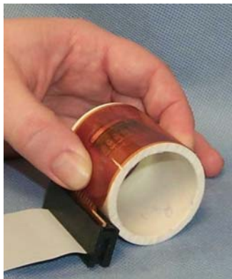
Fig. 7. First-generation sensor calibrated using objects of known curvature
