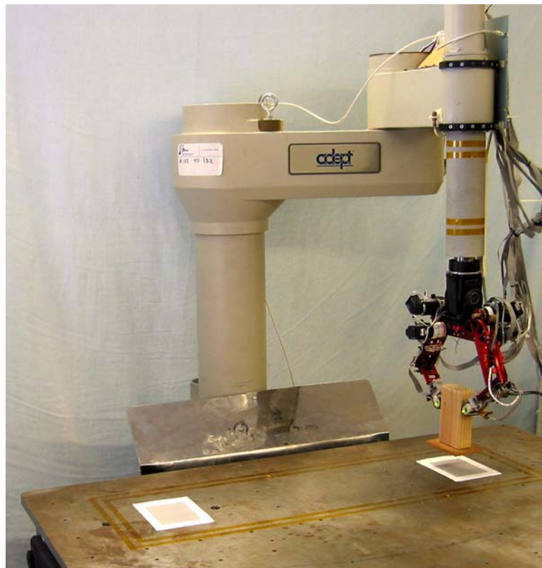
Figure A-1. AdeptOne-MV (SCARA type) robot arm with five degrees-of-freedom. The robot cartesian position and orientation perpendicular to the table are controlled by the operator's wrist position and orientation.
