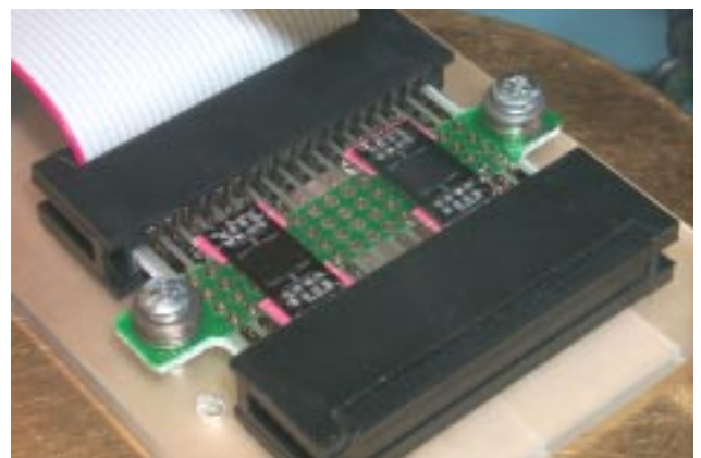
Figure 6: Sensor mounting. Test sensor elements are affixed in pairs to interchangeable printed circuit boards for wire-bonding.
