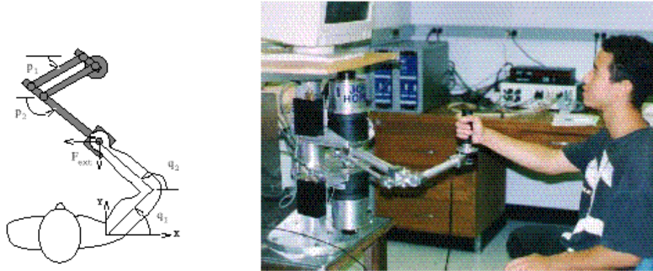
Figure 3. The robotic manipulandum and the experimental setup. The manipulandum is a very low friction, planar mechanism powered by two high performance torque motors. Subject grips the handle of the robot. The handle houses a force transducer. The video monitor facing the subject displays a cursor corresponding to the position of the handle. A target position is displayed and the subject makes a reaching movement. With practice, subject learns to compensate for the forces produced by the robot.
