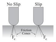
Figure 6: A representation of contact forces, with and without slip.
