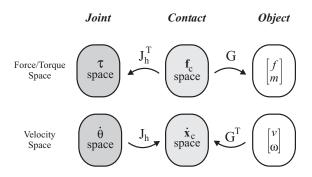
Figure 2: The role of the hand and grasp Jacobians. For the fingers,  $\tau$  is the vector of joint torques and  $\theta$  is the vector of joint velocities. For the contacts,  $\mathbf{f}_c$  is the vector of contact forces and  $\dot{\mathbf{x}}_c$  is the vector of contact point velocities. For the object, the resultant force vector and the vector of object velocities are shown.
