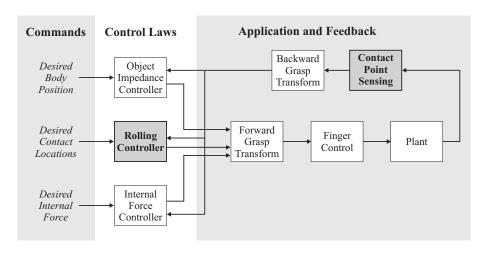
Figure 8: Control block diagram for manipulation with rolling.
